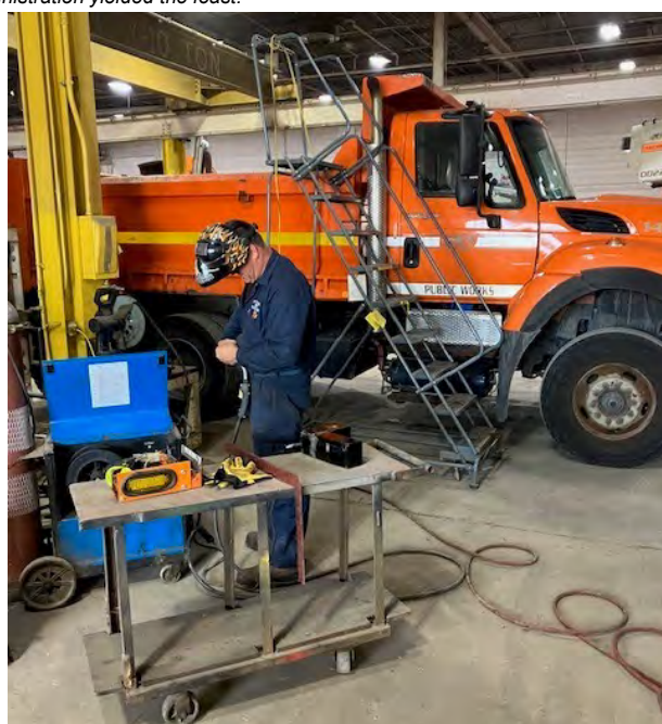
2009 International Dump Truck Welding Repair - Emergency light brackets were re-welded onto the 2009 International dump truck body.
