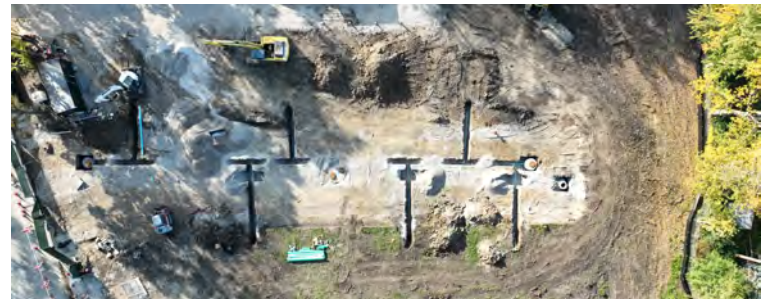
Ponto Court Subdivision Utility Connections (aerial view)
